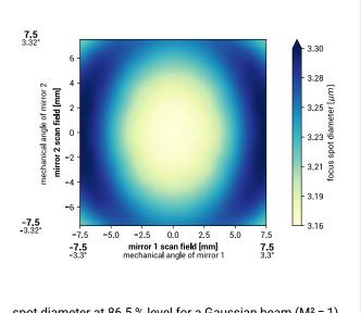
spot diameter at 86.5% level for a Gaussian beam (M² = 1) with 10.0 mm diameter at  $1/e^2$ , clipped at 15.0 mm field size and mirror distances as given above for a two mirror scan system
